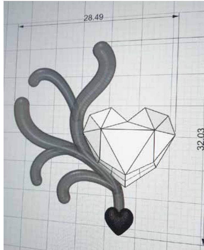
Computer-generated image showing the position of the titanium branches and heart, with the gemstone at the base.
